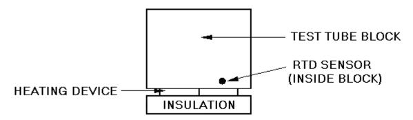
The heating device is in contact with the test tube block at the top and rests on an insulating pad at the bottom. It can be switched on and off many times per second. This fast switching provides the superior temperature stability of the TCON.
